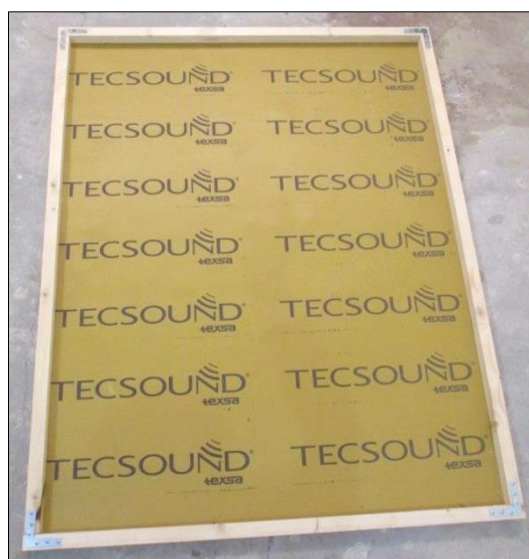
Images 4 to 6 Test element assembly: membrane with wooden frame and perimeter sealing
