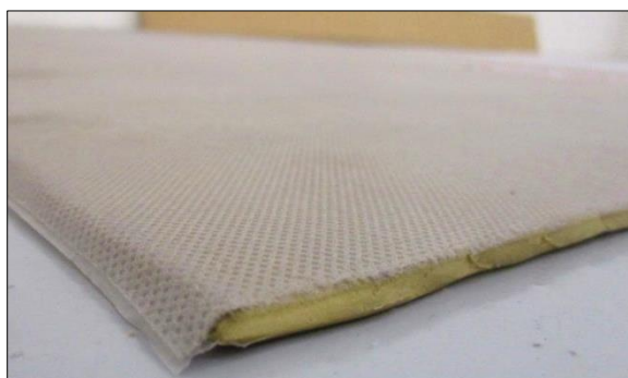
Images 1 to 3 Test element: TECSOUND 100 membrane
